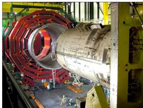
Pict. 2. CMS detector being assembled
